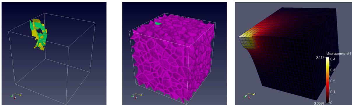
**Figure 11.** Results from the CAFE model on several levels, showing: (left image) micro-cracks in individual grains merging into a propagating macro-crack; (centre image) grain boundaries of a cluster of 1000 grains, and (right) the deformed mesh illustrating the deformation of the body on the macro-scale.
