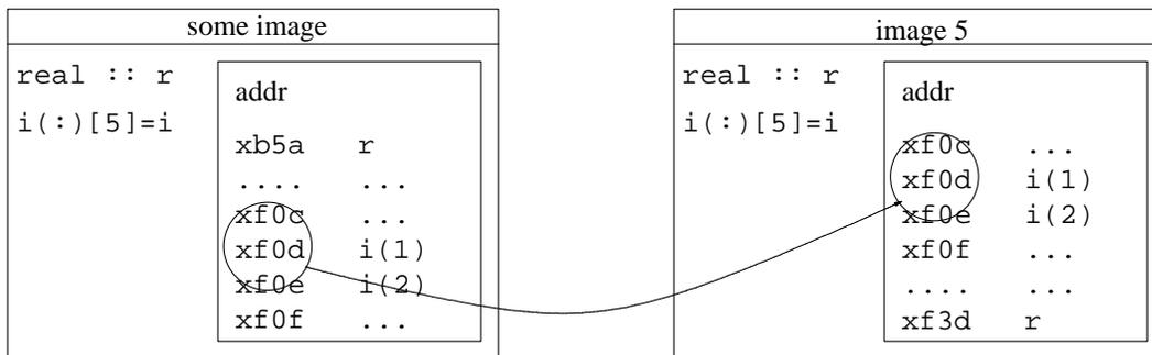
**Figure 1.** A schematic illustration of symmetric memory. On all images coarray variable *i* is allocated at the same address *xf0d*. An ordinary, non-coarray variable *r* is allocated at different addresses on all images.
